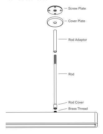
The rod assemblies will arrive packed seperately. A brass thread is fixed to the pendant at the rod locations.
